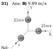
Here,  $P_x = m \times v_x = 1 \times 21 = 21 \text{ kg m/s}$ and  $P_y = m \times v_y = 1 \times 21 = 21 \text{ kg m/s}$
