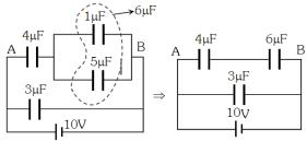
As in series combination, charge remains constant. Therefore, charge across  $4\,\mu\,F$  or  $6\,\mu\,F$  =  $2.4\,x$  10 =  $24\,\mu\,C$
